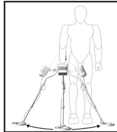
When the stem length is properly adjusted, the 1225-X is balanced for sweeping in a tight semicircle. Always overlap your sweeps by at least 50% or you'll miss a lot of the deeper targets.
