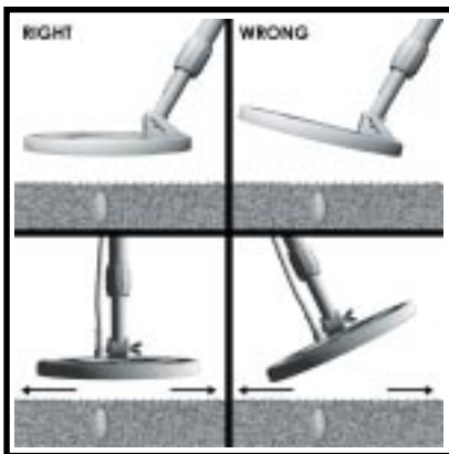
Figure 6. Keep the search coil parallel and close to the ground at all times.
