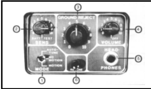
1. **MODE:** This thumb activated switch instantly puts your Gold Bug into one of three operating modes: Auto-Tune, No-Motion or Motion. The Auto-Tune and Motion modes are recommended for searching whereas the No-Motion mode is usually used for pinpointing. For a more detailed discussion, see The section titled "OPERATING MODES".
