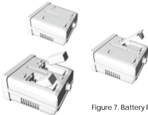
Figure 7. Battery Replacement
