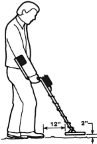
Adjust the stem length and coil angle resting the search coil flat on the ground and about 6 inches in front of your right foot (left foot for left-handers).
