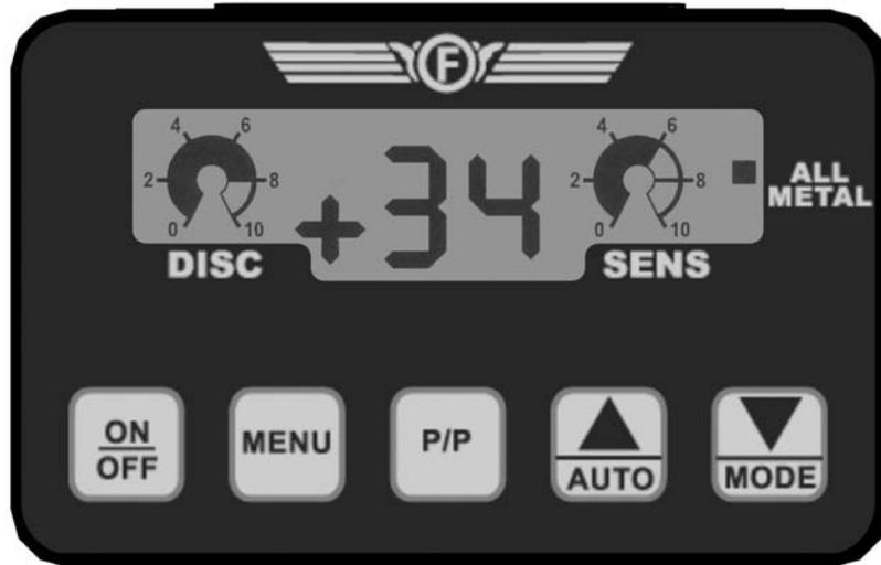
1. The POWER button turns the unit ON and OFF. One of the first things you will notice when you turn on your ID Excel is the battery level display. Fresh batteries will show 9 volts; when the battery level is down to 6 volts, you have about an hour of battery life left. The detector will not turn on if the search coil is not properly connected. This can prove to be a timesaving safeguard.
